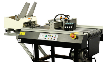
AMS X-JET PRINTER MOUNTED ONTO NORPAK POLYWRAP LINE TO PRINT NAME, ADDRESS, PPI AND RETURN ADDRESS DIRECTLY TO POLYTHENE.
